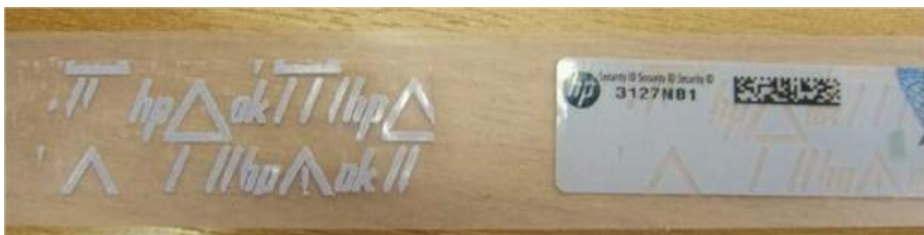
Figure 14: Adhesive left behind on product (left) and signs of tampering on label (right) on previous label
