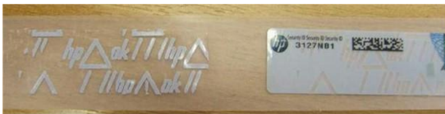
Figure 11: Adhesive left behind on product (left) and signs of tampering on label (right) on previous label
