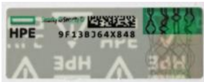
Figure 8: Signs of tampering on current security label
