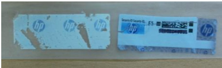
Figure 10: Adhesive left behind on product (left) and signs of tampering on previous label
