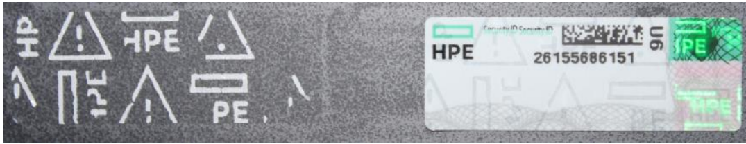
Figure 9: Adhesive left behind on product (left) and signs of tampering on label (right) on previous labels
