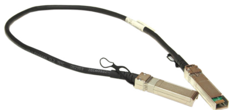
Figure 13: SFP+ DAC cable
