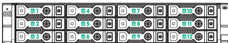
Figure 25 Disk numbering in HPE 3500 and 5100 Systems
