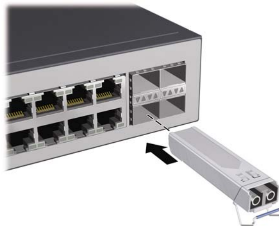
Figure 2-10. Installing an SFP
