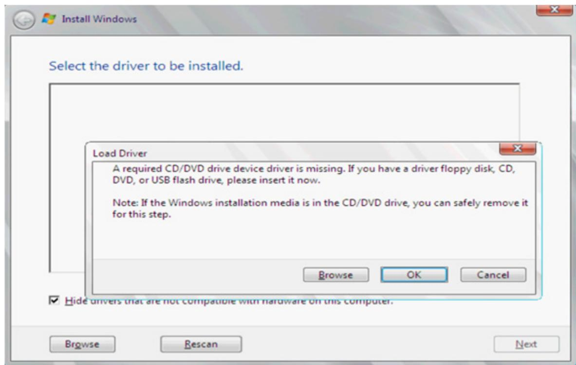
3. For installations that do not use the SATA optical drive to load the Windows installation media, when the "Where do you want to install Windows?" screen appears, click **Load driver**, and then point to the extracted HPE Dynamic Smart Array B140i RAID controller driver folder.
